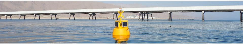
MOBILIS offers a complete range of acquisition data buoys (or smart buoy), perfect support to accommodate all the necessary instrumentation for measurements at sea : sensors, modems, data transmission, technical compartments, wind or solar generators. The larger models are safely accessible and can be visited inside. MOBILIS has developed the expertise of integration and offers two options :
